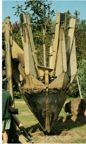
(Left) Tree Spade; (Above) Large percentage of roots removed by tree spade on deeply planted tree.
